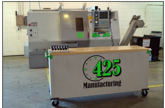
Haas SL30 CNC Turning Center 10" Chuck a Max. part diameter of 28" and a Max. part weight of 500 lbs. when using the tailstock.
