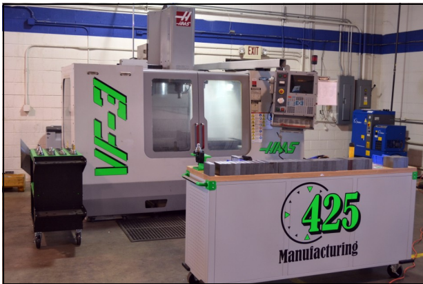
Haas VF-3 CNC Vertical Machining Center X Axis 40" - Y Axis 20" - Z Axis 25" 30 Horsepower and Max. part weight of 3,500 lbs.
